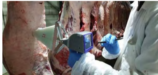
Figure 1 Microwave device developed by Murdoch University
