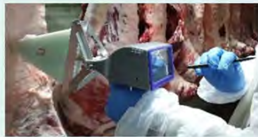
Figure 1 : Measuring fat depth using Microwave Device
